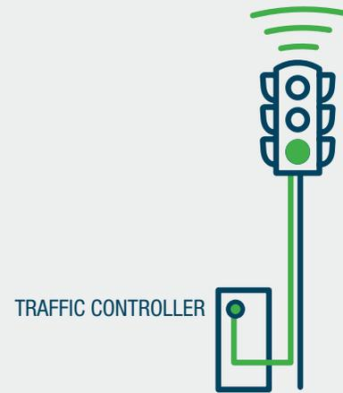
**HOW IT WORKS:** Using its GPS location, Opticom hardware on the vehicle sends a radio signal to the intersection. Hardware at the intersection sends a signal to the traffic controller requesting the green light for the emergency vehicle. When the emergency vehicle passes through the intersection, the traffic signal returns to normal operation. With Opticom Priority Control as a Service, the hardware installation and maintenance are taken care of by GTT as an ongoing service.
